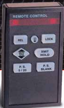
Infrared Cordless Hand Remote Included on Moving Versions
