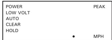
**\*\*WARNING\*\* Never charge a NiCad battery handle until the gun is reading LOW VOLT. Charging any Ni-Cad battery when it is only partially discharged will result in damage to the battery which will substantially decrease the battery performance.**
