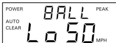
**Hi and Lo Speed Cutoffs** - The upper display indicates the highest speed that the radar will track. The lower display shows the lowest speed the radar will track. By limiting the upper end of the speed range, the Stalker can ignore unwanted signals that occur beyond the speed range. And by limiting the lower end of the speed range, background motion can be ignored. This also helps to increase the sensitivity for objects in the middle of the speed range.
