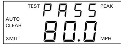
checks calibration. The lower display should read 80.0 mph. A reading of 80.0 mph means the STALKER is perfectly calibrated and it will be accurate throughout the entire speed range. Should your STALKER read any other speed or display FAIL, see the service instructions at the end of this manual.
