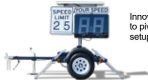
Innovative design allows display to pivot and lock for easier towing, setup, and positioning.
